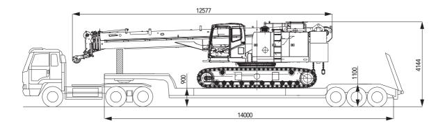
■ Transportation mode II: dismantle the counterweight, jib and lifting hook, transport through two vehicles with maximum weight of single piece transportation 32t and 12.6m x 2.99m x 3.25m (L x W x H)
