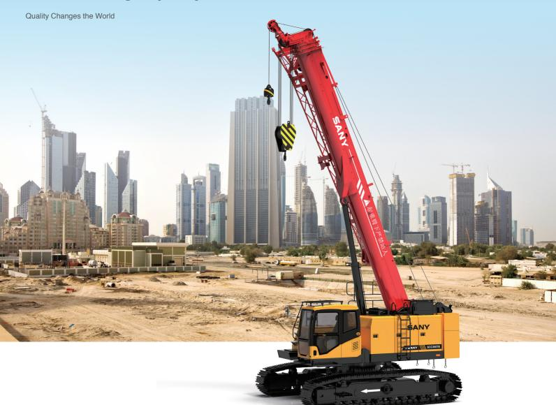
Max. lifting moment: 117.5t⋅m Max. boom length: 31.5m
